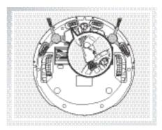
Wipe the Charging Contacts and Charging Dock Pins with the brush of the Multi-Function Cleaning Tool or a dry clean cloth to maintain their effectiveness.
