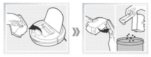
Remove the Sponge Filter and High Efficiency Filter. Pat the High Efficiency Filter clean. Do not rinse the High Efficiency Filter under water.
