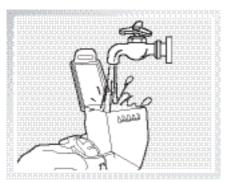
Dry the Sponge Filter, Dust Bin and Filter Net completely before reinstalling.
