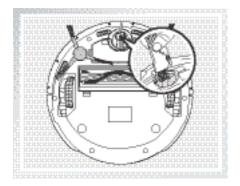
Wipe the Anti-Drop Sensors with the brush or the felt side of the Multi-Function Cleaning Tool to maintain their effectiveness.
