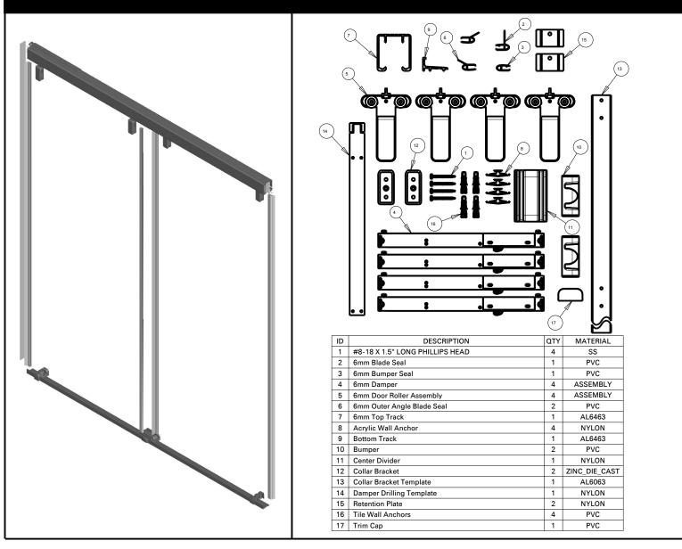
MATERIAL: Anodized Aluminum Extrusions (Track) and Zinc Die Cast (Mounting Brackets). Bronze Finish is Powder Coated.
