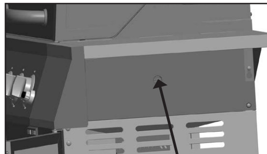
Hole for viewing the flame
