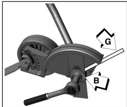
4. Install and center blade (F) on inner blade adapter (B).
