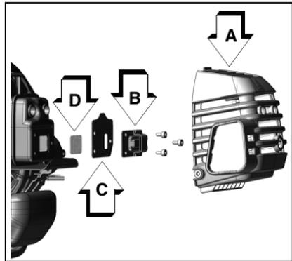
**Note:** When cleaning carbon deposit, be careful not to damage the catalytic element inside muffler.
