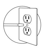
Remove the screw(s) from your outlet face plate using a screwdriver.
