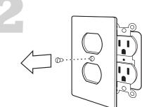
Remove the outlet face place from the wall.
