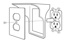
Place face plate over Power Perch. Align face plate and Power Perch to the outlet. Replace face plate screw(s), tightening until Power Perch is secure. Do not over tighten screw(s).
