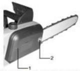
Move the chain tensioning pin to the extreme left hand position by turning the screw counterclockwise as far as it will go.
