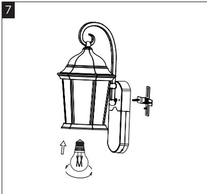
Mount light fixture to long screws as shown, then install both decorative nuts. Install a light bulb
