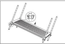
3: Please make sure that you have the perforated steel shelf the correct way up. Hold the perforated steel shelf on its side and slide the top of the four poles through the bottom of the perforated steel shelf at its corners until there is a snug fit. After the four poles have been slid through the perforated steel shelf corner holes, set the perforated steel shelf upright.
