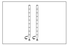
1:Screw the adjustable feet to the one-pice pole.
