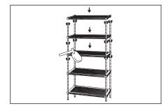
6:Repeat the step(2) and the step(3) to assemble the 3rd and the 4th&5th perforated steel shelf as the photo. Then pushing firmly down on every perforated steel shelf at corners by rubber mallet to sesure the perforated steel shelf in a place over the plastic clips.
