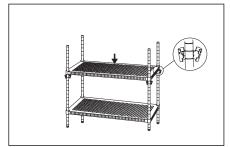
4: Repeat the step (2) and the step (3) to assemble the 2nd perforated steel shelf (A) as the photo.
