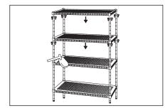
6:Repeat the step(2) and the step(3) to assemble the 3rd and the 4th perforated steel shelf as the photo. Then pushing firmly down on every perforated steel shelf at corners by rubber mallet to sesure the perforated steel shelf in a place over the plastic clips.
