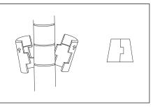
2:Snap the plastic clips into the pole groove of four lower poles at the same position.
