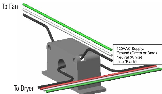
Note: Some 240V AC systems may only have 3 wires, Line 1 (Black), Line 2 (Red) and Ground (Green or Bare). If Lead colors do not match those shown, a Qualified Electrician should identify each lead prior to connection.
