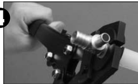
4 Position Crimp Tool jaws over crimp ring and squeeze.
