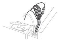
Push the water supply tube into the hole on the top case and pull it through the backplate.
