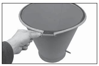
**11.** Remove the lower cyclone separator metal belt using a 10 mm wrench.
