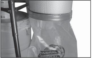
**9.** Fit the plastic collector bag over the bottom of the canister filter.
