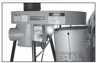
With the help of an assistant, turn the machine upright on a flat surface, then fit the canister against the impeller.
