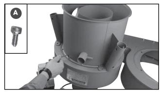
**3.** Attach the cyclone to the impeller using 12 cap screws **A** and a 4 mm Allen key.
