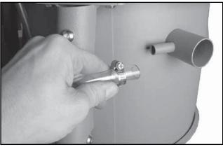
Slide a small hose clamp onto the pressure gauge, and slide the hose onto the fitting at the rear of the impeller.
