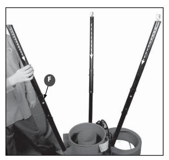
4. Insert the short lower leg into **F** and the two other legs into the other connectors. Twist the legs to align their mounting holes with the corresponding holes in the leg connectors, making sure the legs are leveled, then secure each leg with 4 cap screws per leg using a 5 mm Allen key.
