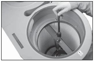
3. Slide the mounting arm onto the canister shaft.
