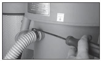
Fit a hose clamp onto the dust hose, and slide the hose onto the fitting. Tighten the hose clamp using a Phillips screwdriver.
