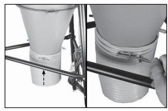
13 Fit a hose clamp onto the junction hose, then slide the hose onto the cyclone. Tighten the hose clamp using a 10 mm wrench.
