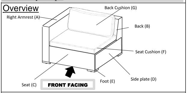
This Right Armchair has multiple parts and may require up to 30 minutes to assemble. To give you an overview of the Right Armchair parts, the above picture is to help you put the various parts into perspective. Please read through the instructions below to familiarise yourself with the parts and steps before assembly.
