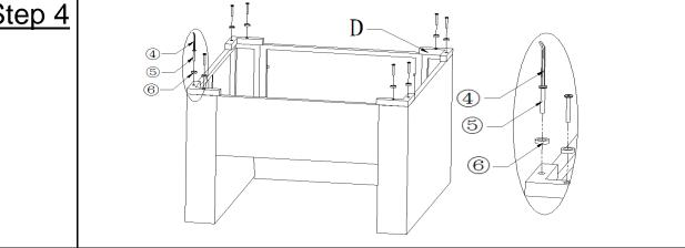
Attach the Feet(D) to the Chair using Bolts(5) and Washer Rings(6) with Allen Key(4).
