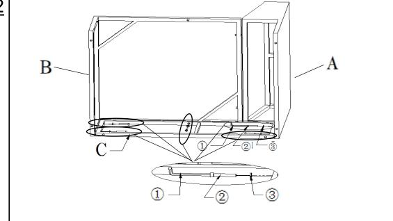
Attach Side Plate(C) between the Chair Back(A) and Chair Seat(B) using Bolt(2) and Washer(③) with Allen Key(1) as shown above.
