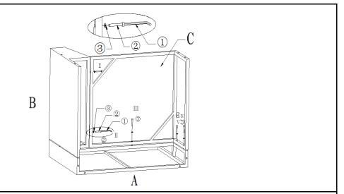
Attach Seat(C) between the Left Armrest(A) and Chair Back(B) using Bolt(2) and Washer(③) with Allen Key(①) from position # I to # V as shown above. Do not fully tigthen.
