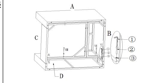
Attach Right Armrest(D) to the Chair Back(B) and Chair Seat(C) using Bolt(2) and Washer(③) with Allen Key(①) from position # VI to # X as shown above. Do not fully tigthen.
