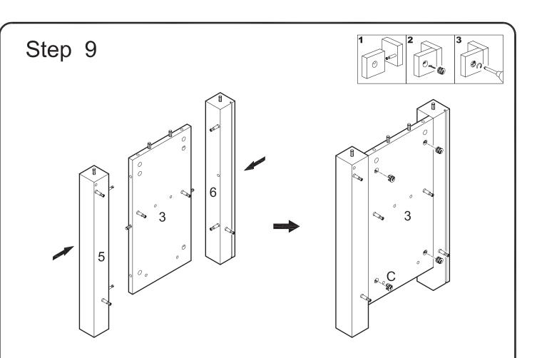
Attach legs (5,6) to panel (3) using cam bolts and dowels as guides. Insert cam locks (C) into panel (3) and tighten with a screwdriver.
