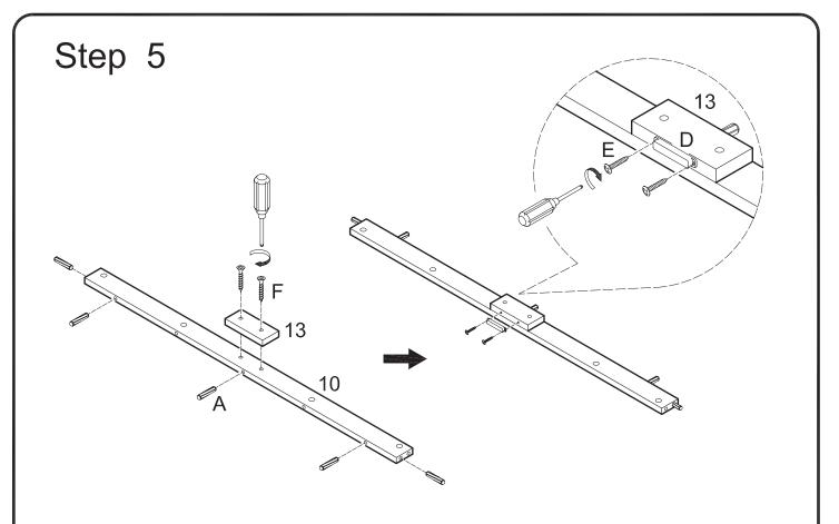
Insert dowels (A) into slat (10). Attach block (13) to slat (10) using screws (F). Attach door stopper (D) to block (13) using screws (E).
