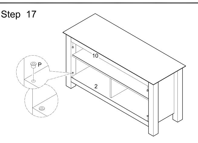
Insert plastic pivots (P) into panel (2) and slat (10).
