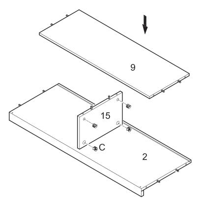
Insert cam locks (C) into panel (15). Attach shelf (9) to panel (15) using cam bolts and dowels as guides. Tighten cam locks (C) with a screwdriver.
