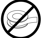
Pipe tape is not recommended.
