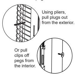
NOTE: New plugs and clips are included in replacement kit. Dispose of used pads, plugs and clips.
