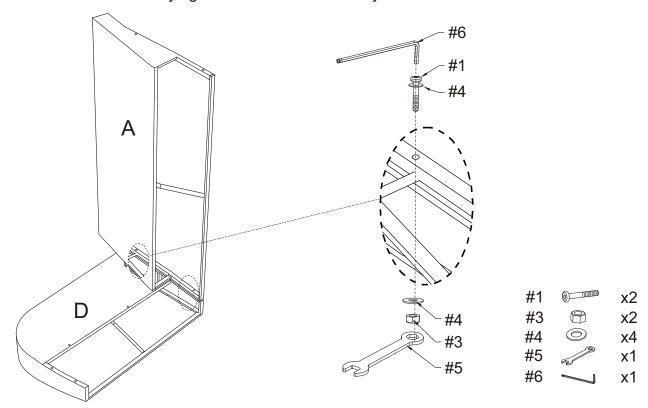
Step 2. Attach seat panel (part B) to back panel (part A) and left arm panel (part D) using short bolts (part #1), long bolts (part #2), flat washers (part #4), hex nuts (part #3), wrench (part #5) and allen wrench (part #6).
