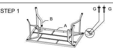
Place table top frame (A) on the ground, then screw table legs (B) to it. Please do not tight any screws to the end at this step.
