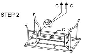
Screw table leg support ring (C) to table legs. Make sure all screws are inserted properly and tighten all screws to the end.
