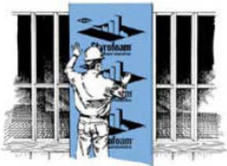
5. Secure Dow insulation boards using 1 3/4" ring shank nails or staples with a 1" diameter plastic cap or equivalent fastener long enough to penetrate framing a minimum of 3/4". Nails or staples should not be over-driven. Secure the 4'x 8' and 4'x 9' boards 12" o.c. around the perimeter and 16" o.c. in the field or as required by the code authority having jurisdiction. Secure 2'x 8' boards 12" o.c. on each stud (3 fasteners per stud) or as required by the code authority having jurisdiction.
