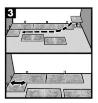
8. Start the third row with the tile cut at 1/3 of a length (8"). Again the remaining piece can be used at the opposite end of the row, if the layout of the room permits.
