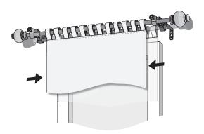
6 Lock rods into position by tightening leveling screw by hand until finger tight. this will prevent the rod from moving.
