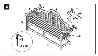
Step 4 : tighten back (A) with Allen Screw S (H4) and Allen screw L (H3) as shown on picture. Tighten with the Allen key (H8). Put the seat (G) to the bench.
