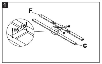
Step 1 : attach support (B) to front (F) and long bar (C).Using screw S (H6) and tighten with the screwdriver as shown on the picture.
