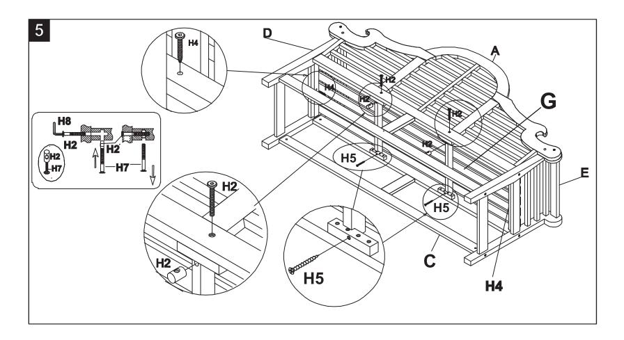
Step 5 : tighten seat (G) with bolt S (H2) and screw L (H5) as shown on the picture.
