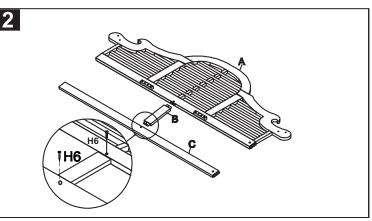
Step 2 : attach support (B) to long bar (C).Then attach it to the back (A) as shown on the picture . Using screw S (H6) and tighten with the screwdriver.
