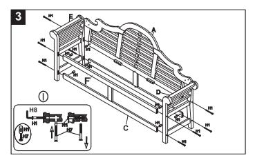
Step 3 : attach the left side (D) and the right side (E) to the back (A) and front part (F) by using the bolt L (H1). Tighten with the Allen Key (H8) as shown on the picture(I).
