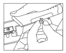
ATTENTION: The Ratchet Modular Plug Crimper cannot be released when tension is too high. To release crimp tool, turn release screw in a counterclockwise direction.
