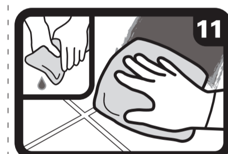
Lightly clean off excess mortar with damp sponge CAUTION: Do Not Over Water
