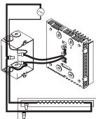
3 Push any excess wire back into the electrical box.
