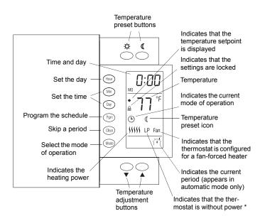
\* LP appears only for the first two minutes when the thermostat is without power. This can occur during a power outage or when the thermal protection device inside the base-board heater is opened.
