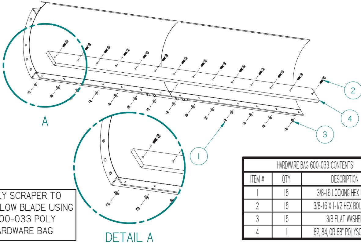
ATTACH POLY SCRAPER TO FRONT OF PLOW BLADE USING SUPPLIED 600-033 POLY SCRAPER HARDWARE BAG
