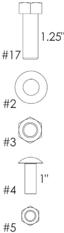
USE HEX BOLTS, WASHERS, AND LOCK NUTS TO ATTACH BLADE TOGETHER
