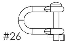
THREAD END OF CHAIN ONTO SHACKLE AND ATTACH TO PASSENGER SIDE WINCH ARM.
