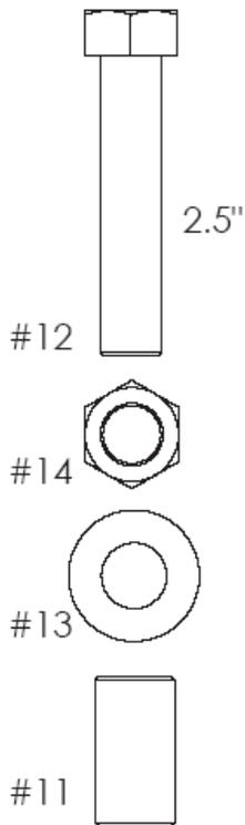
CONNECT UPPER AND LOWER A FRAMES USING HEX BOLT, SLEEVE, WASHERS, AND LOCK NUT
