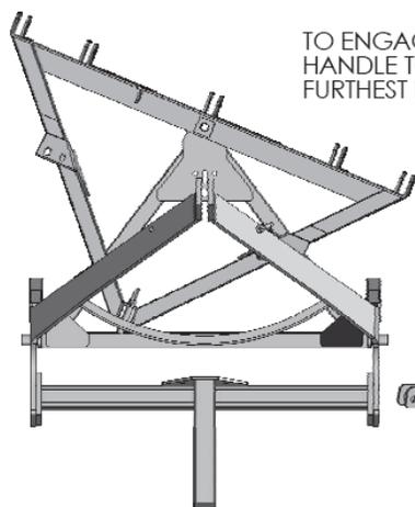
TO ENGAGE SAFETY CHAIN USE RELEASE HANDLE TO MOVE UPPER A-FRAME TO FURTHEST DRIVER SIDE SLOT.
