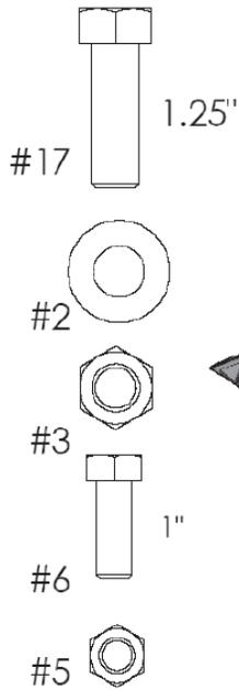
USE HEX BOLTS, WASHERS, AND LOCK NUTS TO ATTACH BLADE TOGETHER
