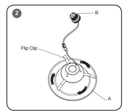
STEP 1: Carefully rotate the "Flip Clips" clockwise until the clips are fully-deployed. See Figure 2.
