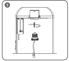
**NOTE:** For 5" recessed cans, it is recommended not to rotate the flip clips into the fully dep loyed position.
