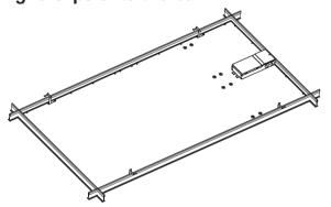
Remove the cover of junction box on the back of the fixture with a screwdriver. Remove the knockouts on the A and B side with a screwdriver.
