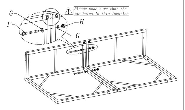
Secure the seat base-left(C1)to the seat base-right(C2) using screws(F)and flat washers(G)and nuts(H) in two places.
