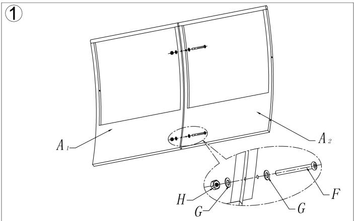
Secure the seat back-left(A1)to the seat back-right(A2) using screws(F)and flat washers(G)and nuts(H) in two places.
