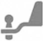
**Hitch:** A device on the tow vehicle, to which the coupler of the trailer is attached. The hitch also supports the weight of the trailer tongue.
