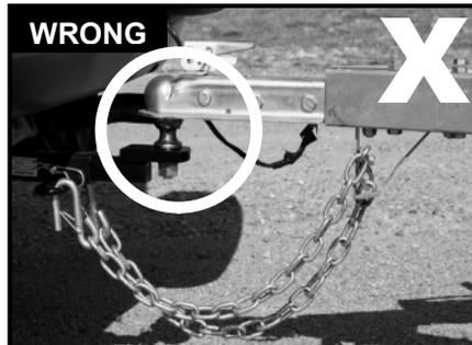
**The coupler latch must always be closed when towing the trailer!**
