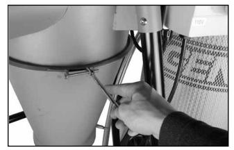
**12.** With the help of an assistant, hold the lower cyclone against the upper cyclone and tighten it over the joint between the 2 sections to hold them together using a 10 mm wrench.
