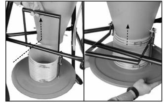
19. Pass the handle under and behind the front cross brace. Slide the hose back onto the cyclone, then tighten the hose clamp.
