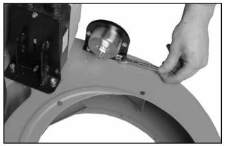
2. Attach the pressure gauge to the impeller with the flange bolts you just removed.
