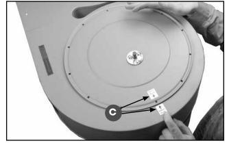
5. Place the canister lid on the impeller with the mounting arm through the center hole. Align the reference marks **C**.
