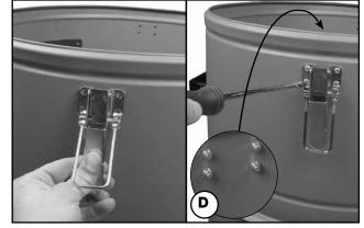
8. Align the latch mounting holes with the holes in the drum. Attach the 2 latches to the drum using phillips screws with and nylock nuts inside the drum **D**.
