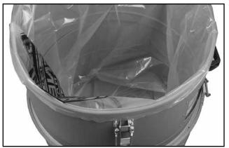
9. Install the liner bag (the bigger of the 2) inside the drum.
