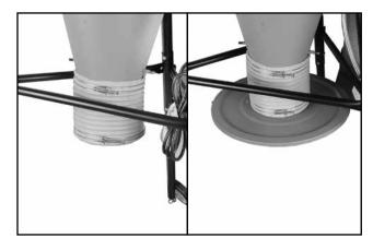
**15.** Fit the other hose clamp onto the opposite end of junction hose. Slide the fitting on the drum lid drum lid into the junction hose, and tighten the hose clamp.
