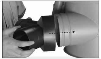
1. Slide the hose fitting onto the inlet.
