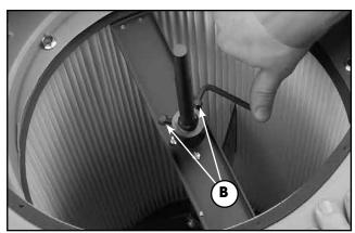
4. Secure the arm by tightening screws **B** using a 5 mm Allen key.
