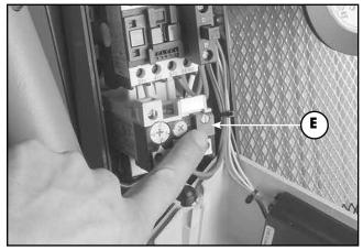
Press on the button E to reset the overload protection. Re-install the cover and then retighten the two screws D before starting the machine.
