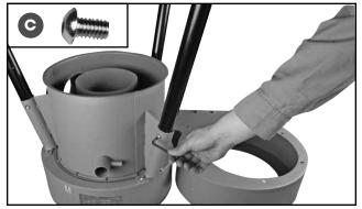
Align the leg mounting holes with the corresponding holes in the bracket, then secure each leg with 3 cap screws per leg C using a 5 mm Allen key.
