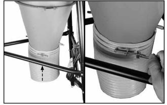
**13** Fit a hose clamp onto the junction hose, then slide the hose onto the cyclone. Tighten the hose clamp using a 10 mm wrench.
