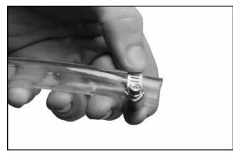
3. Slide a small hose clamp onto the end of the hose.
