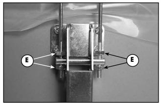
Note: If needed, adjust the nuts and jam nuts **E** so that the latches firmly close the lid.
