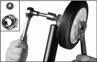
2. Attach the wheels by tightening the nylock nut A using a 19 mm wrench and an adjustable wrench.
