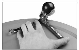
**3.** Lock each swivel caster by tightening the jam nuts with two 12 mm wrenches.
