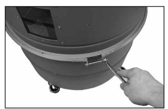
6. Slide the metal belt down over the top drum and tighten it over the joint between the 2 drums to hold them together.
