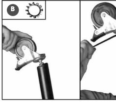
Screw the lockable swivel caster with a sprocket washer B into the short leg, then secure it in position by tightening the two jam nuts using two 14 mm wrenches.
