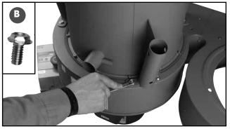
4. Complete the assembly using 6 flange bolts **B** and a 12 mm wrench.
