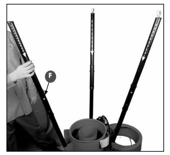
4. Insert the short lower leg into **F** and the two other legs into the other connectors. Twist the legs to align their mounting holes with the correponding holes in the leg connectors, making sure the legs are leveled, then secure each leg with 4 cap screws per leg using a 5 mm Allen key.
