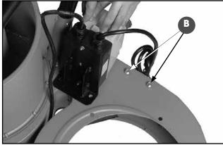
1. Using a 10 mm wrench remove the 2 flange bolts B.
