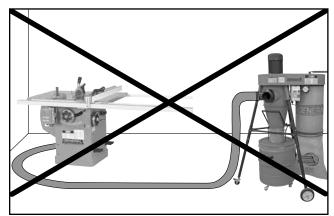
Wherever possible avoid running hoses and ducting along the floor.
