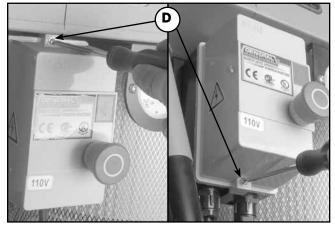
1. Loosen the two screws **D** with a Phillips screwdriver until you can remove the switch cover.
