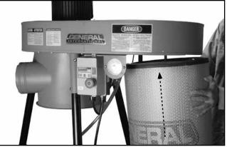
1. With the help of an assistant, turn the machine upright on a flat surface, then fit the canister against the impeller.
