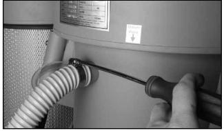
**3.** Fit a hose clamp onto the dust hose, and slide the hose onto the fitting. Tighten the hose clamp using a Phillips screwdriver.
