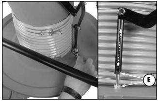
23. Adjust the height of the arms as needed, then tighten the nuts **E** as shown: one against the lid and the other against the draw bar.
