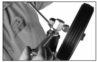
**3.** Secure the wheels in the proper position by tightening the jam nuts using two 14 mm wrenches.
