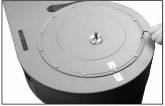
7. Once all the screws are installed, tighten them all the way for an airtight seal.
