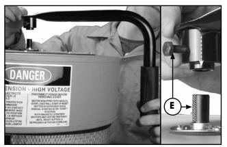
8. Fit the handle onto the mounting arm, making sure the bolt is aligned with the flat side of the arm. Then secure it in place with the bolt **E** using a 10 mm wrench.
