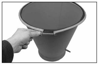
11. Remove the lower cyclone separator metal belt using a 10 mm wrench.
