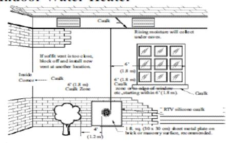
AWARNING: Moisture in the flue gas will condense as it leaves the vent terminal. In cold weather this condensate can freeze on the exterior wall, under the eaves and on surrounding objects. Some discoloration to the exterior of the building is to be expected. However, improper location or installation can result in severe damage to the structure or exterior finish of the building.
