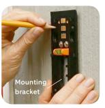
Snap the provided level onto the mounting bracket and use it to help position the bracket.
