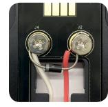
If you have a **digital doorbell**, connecting the diode the wrong way won't do any harm. If your doorbell doesn't ring, just reverse the diode.
