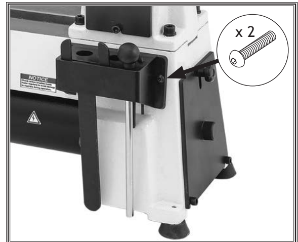
Figure 11. Tool holder attached to bed.
