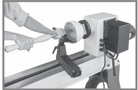
Figure 28. Typical faceplate turning operation.
