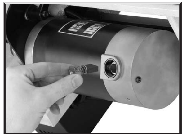
Figure 43. Removing brush from motor.
