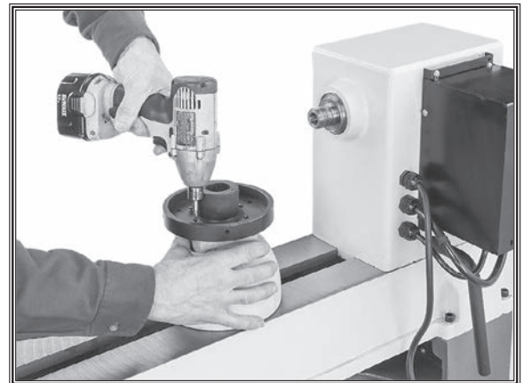
Figure 29. Typical attachment of faceplate to workpiece.
