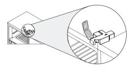
3 Press the refrigerator door open detection switch 5 times as in the figure to make the light inside the compartment
