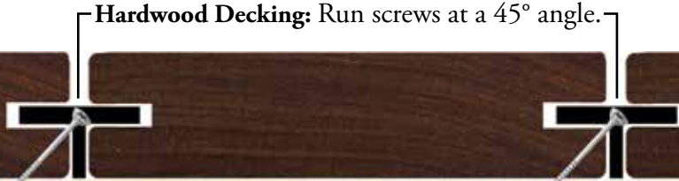
Shown Above: Ipe (Brazilian Walnut) Hardwood decking installed with DeckWise® Extreme™ hidden deck fasteners.
