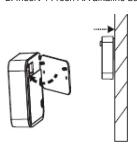
5. Slide light onto mounting bracket attached to wall.
