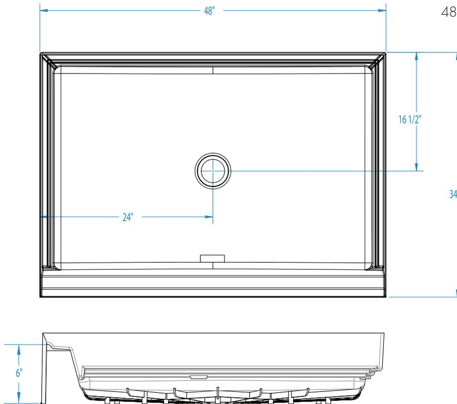
**FEATURES** lbs (kg) Dimensional Tolerance  $\pm \frac{3}{16}$ ". Dimensions needed for site preparation should be measured from the unit. Aquatic assumes no responsibility for preparatory work.
