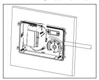
5. Replace the lens set on the hinge and finish connection, Close the lens set and tighten the screws to fasten the lens set to the back plate.
