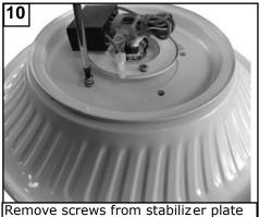
Remove screws from stabilizer plate on bottom of fan motor.
