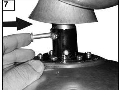
Insert downrod into motor yoke. Next, insert clevis pin through yoke and downrod.
