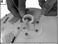
Remove keeper from pin. Remove pin, replace keeper and save.
