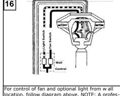
location, follow diagram above. NOTE: A professional electrician is recommended for this type of installation.
