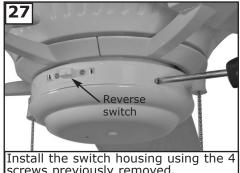
Screws previously removed. Setting the reverse switch in the left hand side will result in downward airflow and setting the switch in the right hand side will result in upward airflow.
