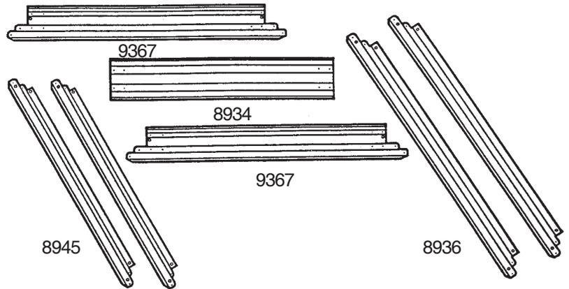
**1** Place the **front floor frames** as shown. Center the **ramp**, with drain holes facing outside, on top of the two front floor frames. Join the frames by inserting eight screws.
