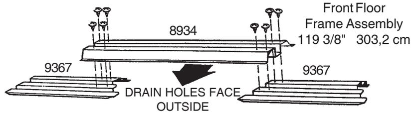
**2** Overlap the **side floor frames** and the **rear floor frames** as shown. The holes in these pieces will align when the pieces are positioned with correct amount of overlap. See the illustrations below for the proper overall length of the side and rear floor frames. Join the frames by inserting five bolts into each frame set as shown.
