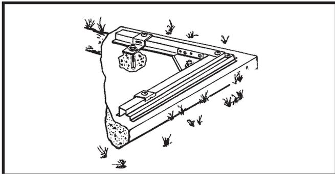
**Anchoring into Concrete:**
