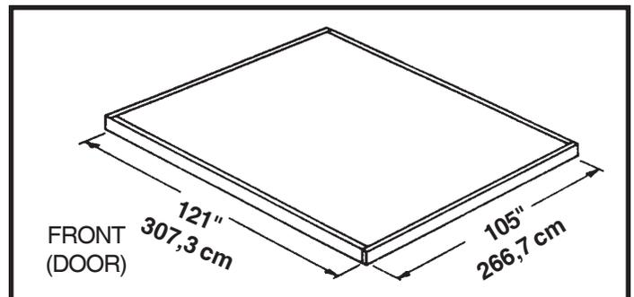
Note: Finished Slab dimensions, with lumber removed.
