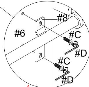
2) Align shelves (#3,4,5,6) to the fixed plates of the frames as shown in the diagram, then secure by using bolts (#C).
