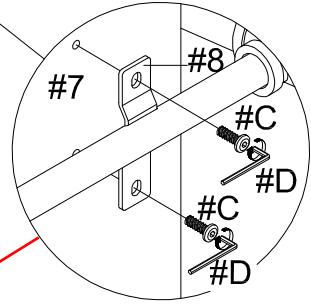
2) Align bottom shelf (#7) to fixed plates (#8), then secure by using bolts (#C).
