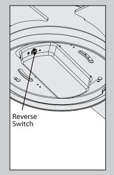
**To switch the direction of air flow,** move the reverse switch to the opposite position. You will need to remove the glass to do so.
