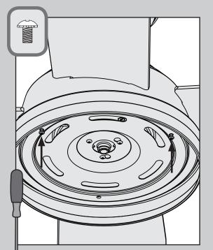
Screw two housing assembly screws from the  $\equiv$  hardware bag halfway into the  $(\mathbf{X})$ upper switch housing. It does not matter which two screw holes you choose.
