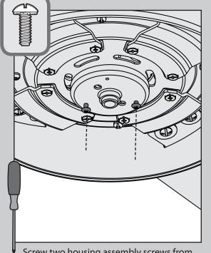
Screw two housing assembly screws from
