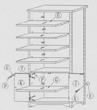
the holes of door (K/J) and rotate the screws (X through the middle holes of door (K/J) into the knob (V). Finally, put the shelf (G) onto the shelf support (W). (See the left picture).
