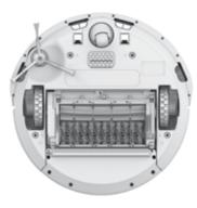
Important: A front wheel clogged with hair and debris  $\swarrow$  could result in floor damage.
