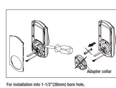
simply pry the adapter collar off with a screwdriver
