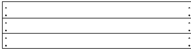
RP2 - ROOF PANEL - W2A01771 (2) 1 5/8"x15 5/8"x63 3/4" (42x396x1618)
