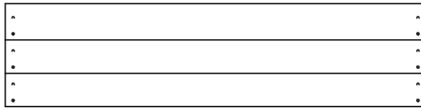
RP2 - ROOF PANEL - W2A01771 (2) 1 5/8"x15 5/8"x63 3/4" (42x396x1618)
