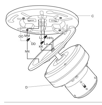
If you wish to install an optional wall control, use this diagram as a guide but refer to the installation manual for the wall control for the correct color and wire connections.
