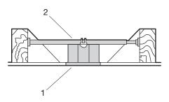
To hang your fan where there is an existing fixture but no ceiling joist, you may need an installation hanger bar (2) (not included) as shown above.
