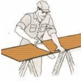
If measured floor-to-ceiling height is 8' or less, subtract  $\frac{1}{2}$ " from this measurement to allow  $\frac{1}{4}$ " expansion clearance on top and bottom. Transfer these measurements to panels for cutting. If using a handsaw or table saw, mark and cut the panels face up. If using a portable circular saw or sabre saw, mark and cut panels face down. Cut-outs for door and window sections, electrical switches and outlets or heat registers require careful measurements.
