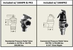
**Specifications:** Designed for residential or commercial use with potable water. This approved Webstone valve is actuated by a blowout proof stem and features an adjustable packing gland. Solder joint temperature ratings are per ASME B16.18 Annex A for 95-5 solder. Other solder materials have lower pressure/temperature limits. Do not silver braze or overheat valves when soldering.
